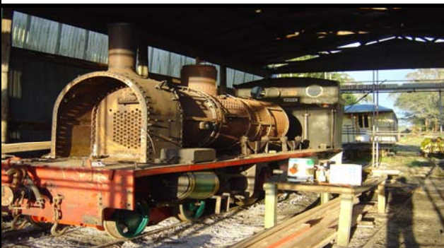
Gabriel –bares it all for the future.. Nice new shoes but she is stripped for the boiler inspection etc.
